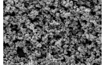
The photocatalytic coating has been developed by the University of Bath to provide a product which can be applied to indoor surfaces in order to neutralise Volatile Organic Compounds (VOCs) and therefore promote a healthier indoor environment. The coating is applied to a substrate by painting, rolling or spraying, and comprises titanium dioxide (anatase) particles bonded to the substrate by a polyurethane/acrylate polymer.
